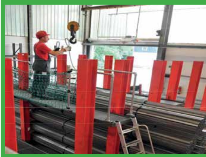
Safe access for attaching lifting hooks.
