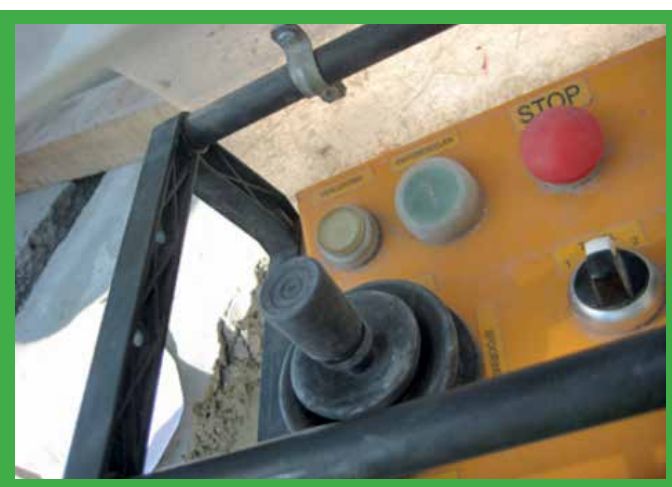
Dead Mans Joystick. You must push down to activate the joystick.
