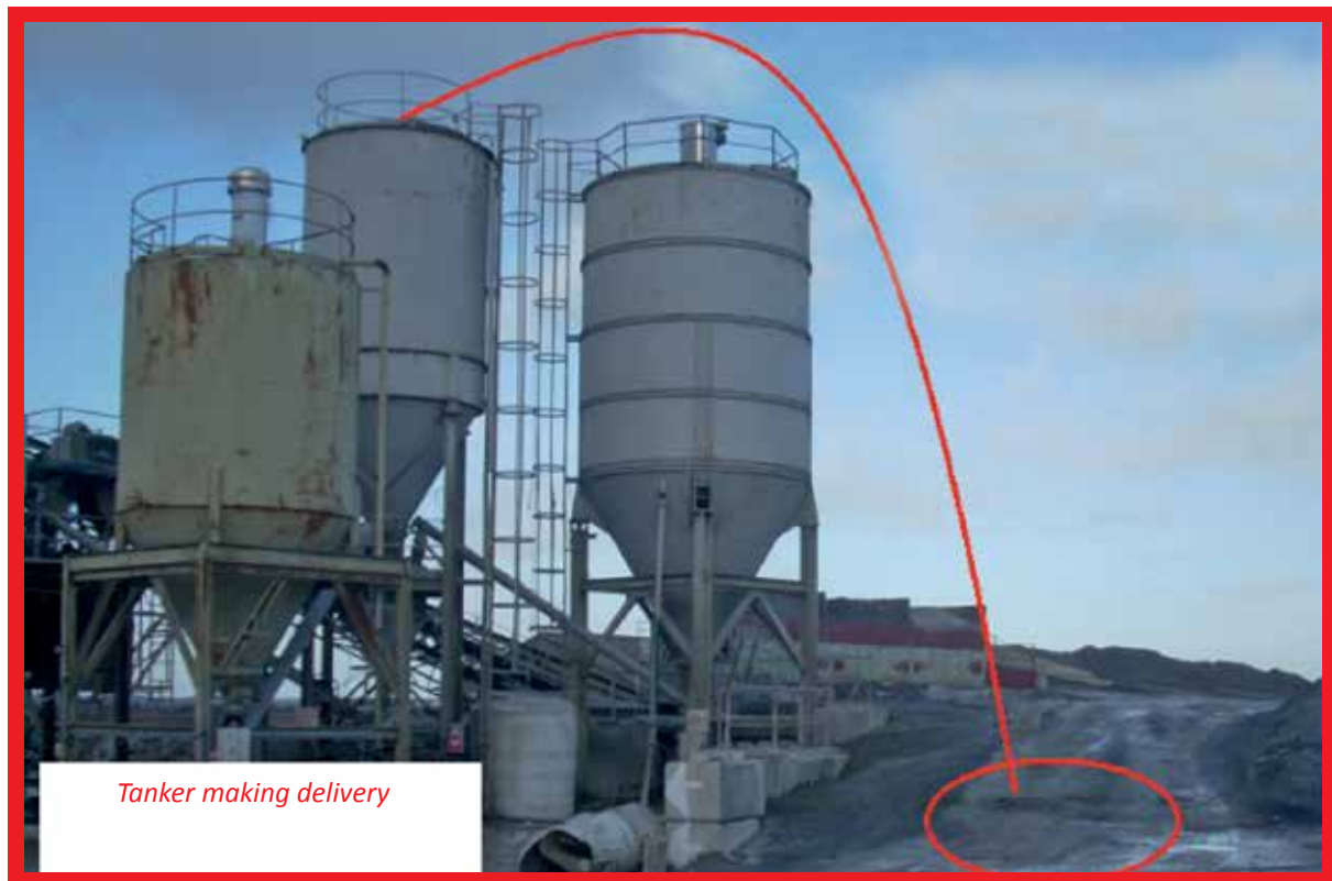
Incident - Near Miss 2012: Filter blown onto nearby area
